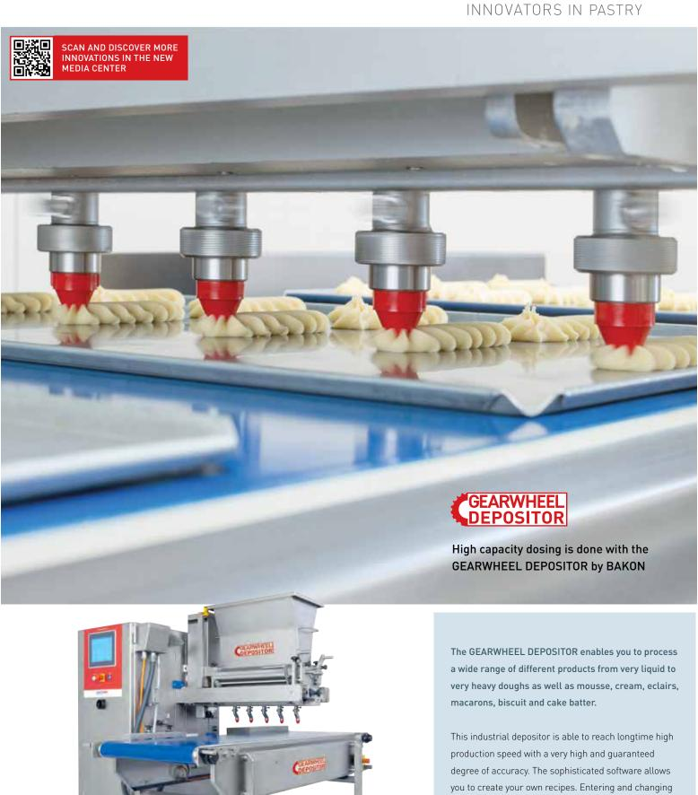
This industrial depositor is able to reach longtime high production speed with a very high and guaranteed degree of accuracy. The sophisticated software allows you to create your own recipes. Entering and changing various parameters is easily done by using the 10 inch full colour touch screen. The GEARWHEEL DEPOSITOR is available in different models and extendable with a large number of options.
