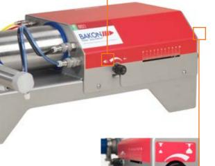
Dosing volume | The dosing volume is manually set and indicated on the scale
