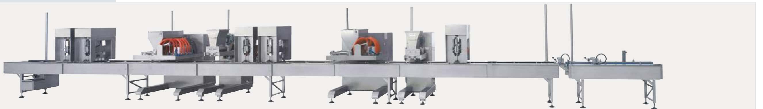
Complete production line with integrated Gearwheel Depositors
